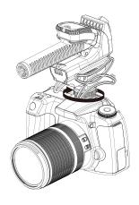
Tighten the thumb wheel by turning it counter-clockwise to secure the microphone. WARNING: Do Not Overtighten!
