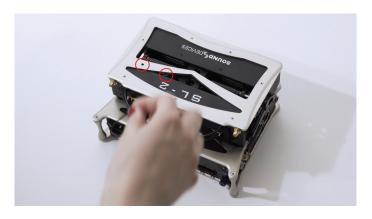
STEP 2 Insert the allen wrench into these holes, visually confirming that the wrench is in contact with the safety screws inside the SL-2. Turn the wrench counterclockwise to loosen the screws. Remove the screws and set aside.
