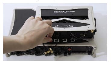
**STEP 8** Secure the SL-2 to the Scorpio Front Bracket with two 6 mm screws using the supplied 2 mm Allen Wrench.
