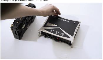
**STEP 5** Replace the originally provided rear black screws near the Sound Devices logo using #4 Phillips head screwdriver.
