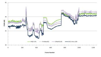
Figure 8 – PSNR comparison of 8:1 class codecs.
