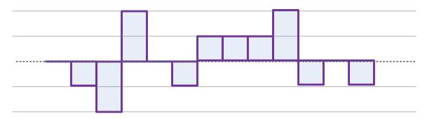
Figure 3 – Noise added by 8-bit quantization of 10-bit signal.
