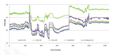
Figure 7 – PSNR comparison of 5:1 class codecs, and HQX at 3:1.
