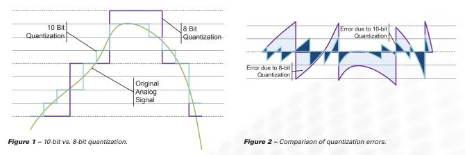
Quantization is performed by capture devices such as cameras or field recorders, which are increasingly capable of capturing pictures with at 10-bit precision. The quantization errors (or noise) introduced by the capture device are unavoidable, but only happen once. What does this have to do with the Intermediate Codec used? The answer is whether or not a second, much noisier set of errors is introduced when an 8-bit Intermediate Codec is used to compress a 10-bit signal.
