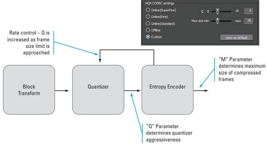
Figure 5 – HQX codec architecture.
